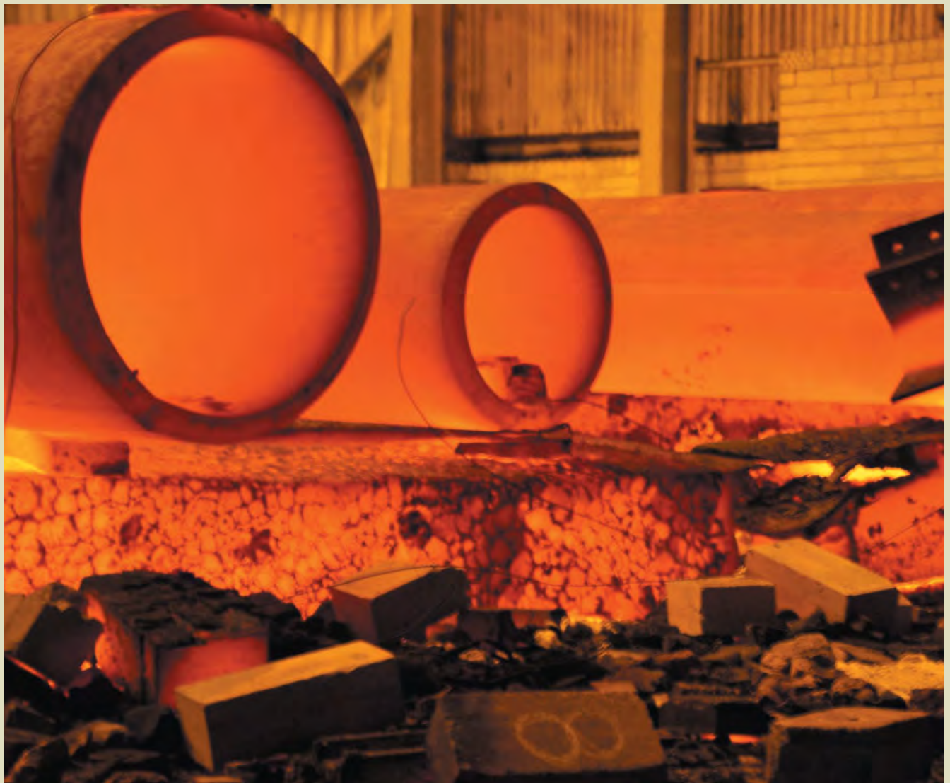
Figure 7: Manipulation of material property. Primary leg elements undergoing heat treatment.
