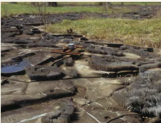
An analogue model of the entire Mississippi basin made by German Pows (mostly generals from the Afrika Korps) at a scale of 1 foot:1 mile horizontally, 1:800 vertically and 5 minutes for a day. It was used until computers took over in the early 1990s to simulate storm bursts as they happened and thus predict the priority of relief provision.
