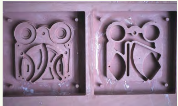
Pattern for Cold Bog diorama camera. The left-hand side is the top, and shows the plan of the film plane. The underside is on the right where the wind-on film-holding-mechanism pockets are visible.
