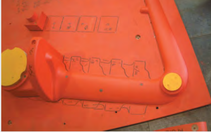
Timber pattern of the stainless-steel castings of the Ballingdon Bridge balustrade showing, by drawing, the variation in the casting length responding to the curved form of the precast-concrete superstructure
