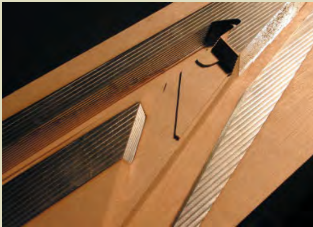
The tacit component and the numerically controlled model. Forming and postforming experiments by the author on the use of CAM as an incremental and interrogative method within an iterative design process. Alloy cast within hardwood section and milled.
