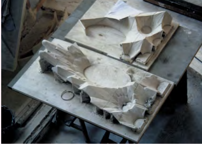
The interior and exterior of the Sagrada Família Church clerestory windows, as proposed by Gaudí at a scale of 1:10.
