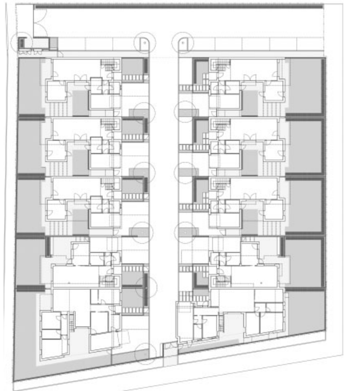
The row of buildings facing the countryside consists of two units of five houses. The first three houses have the same floor plan, which is mirrored in the fourth house. The last house has a patio layout on a single floor that opens to the countryside. The ground floor adds some single-storey volumes that help define a small courtyard in front of the houses.
