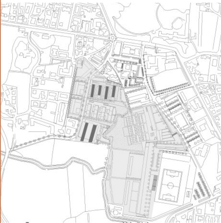
The project includes three rows of residential blocks, one of which is subsidised housing, with the heights and densities of the blocks decreasing towards the countryside. Within the scheme, pedestrian and vehicle entrances are differentiated. Contrary to usual practice, the high-density building is located near the historic centre.
