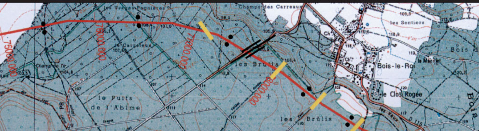
The overpasses in the Solognote forest on motorway A85 between Angers and Tours (1993–7) were designed and planted to minimise disruption by the motorway of forest paths used by wildlife.
