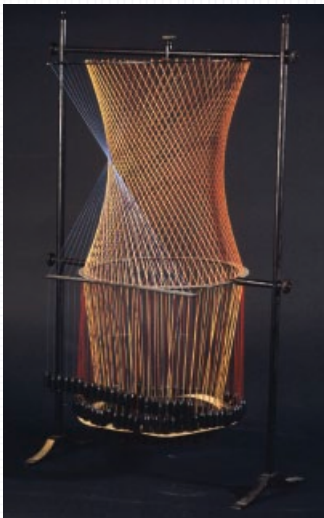
Figure 5. Model of hyperboloid of revolution A parametrically variable analogue model of a hyperboloid of revolution. The most recognisable hyperboloids of revolution are cooling towers of power stations.
